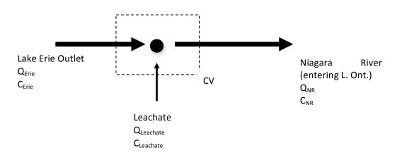
Assume Niagara River serves as a node. Nodes must be at steady state has they have no volume or capacity to store. Meaning nodes cannot accumulate either positively or negatively. Thus, Steady State is assumed.
